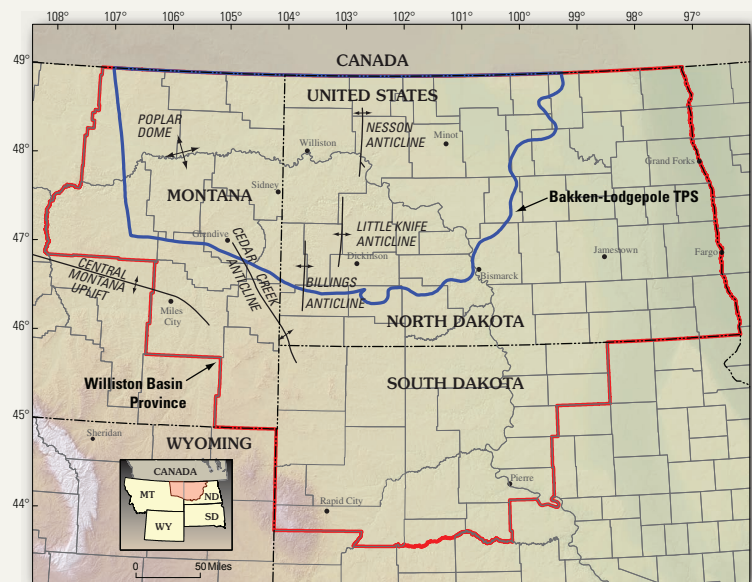
Figure 1. Map showing Williston Basin Province boundary (in red), Bakken-Lodgepole Total Petroleum System (TPS) (in blue), and major structural features in Montana, North Dakota, and South Dakota.
